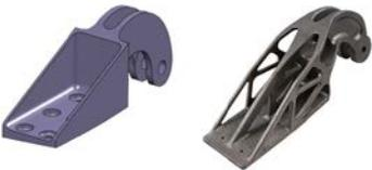
***Figure A.1 Shape optimization in additive manufacturing***
